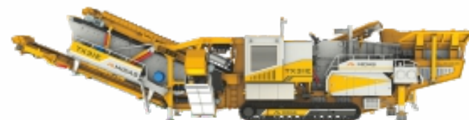
TRACKED MOBILE IMPACT CRUSHING AND SCREENING STATION
